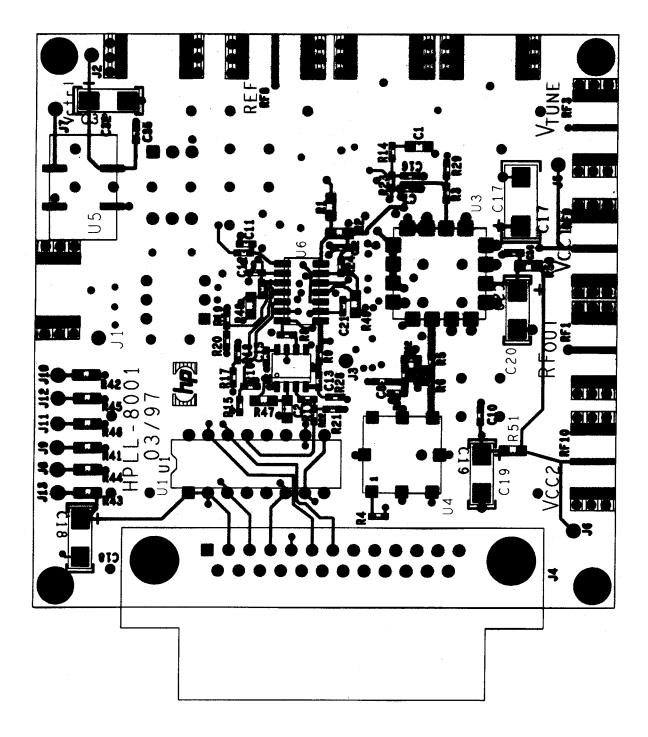
Figure 3. Demo Board PCB Layout
