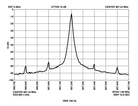
Figure 4. Typical GSM Spectrum Plot
