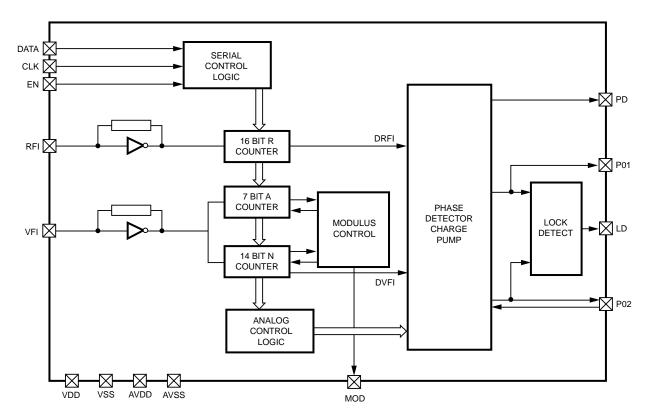
Figure 1. HPLL-8001 Internal Block diagam
