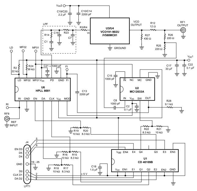
**Figure 2. PLL Frequency Synthesizer Schematic**
