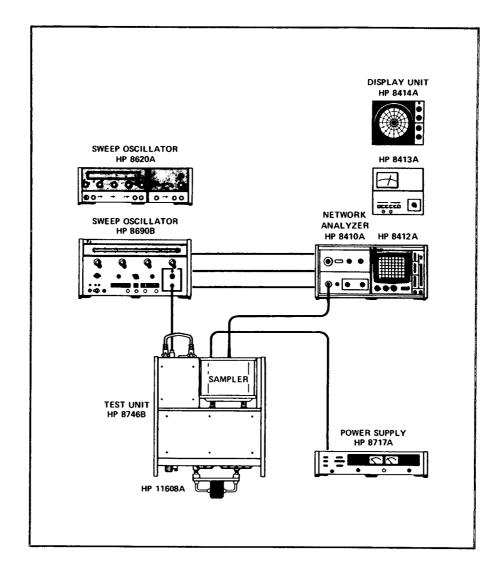
Figure 3. System Configuration for Stripline Measurements
