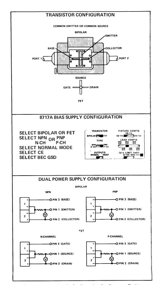
Figure 11. Bias Supply Configuration for Common Emitter
