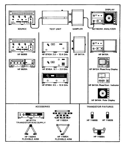
Figure 1. Network Analyzer System Components
