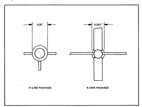
Figure 6. TI-Line and K-Disc Package Styles
