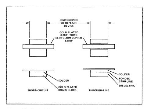
Figure 17. Typical Short Circuit and Through Line Calibration Units
