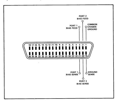
Figure 9. Bias Connections to the 8746B Rear Panel Connector
