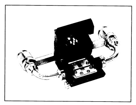
Figure 7. The 11608A Transistor Fixture
