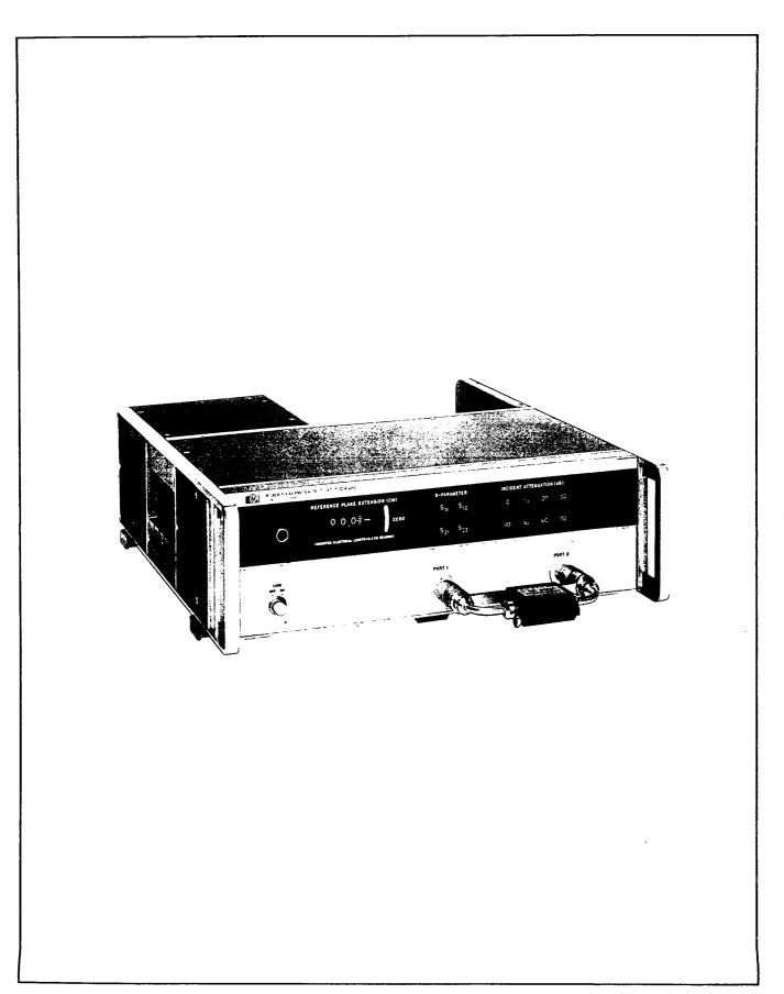
The 8746B S-Parameter Test Set and 11608A Transistor Fixture
