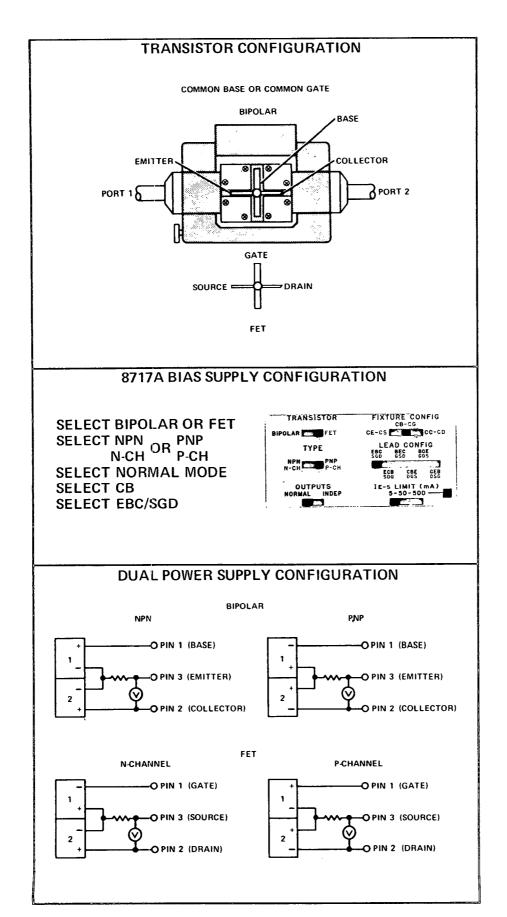
Figure 12. Bias Supply Configuration for Common Base
