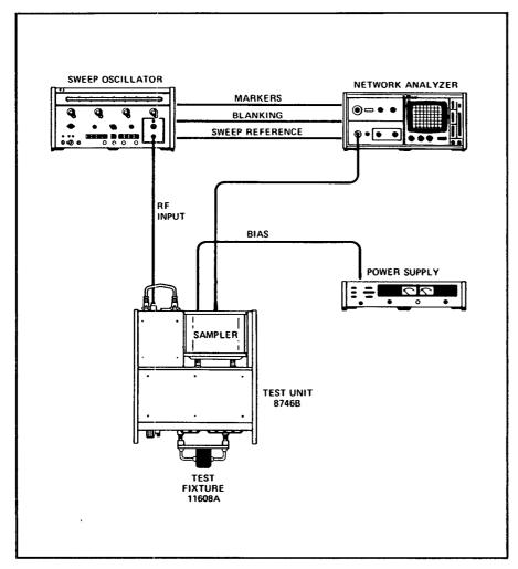
Figure 14. System Interconnection Diagram
