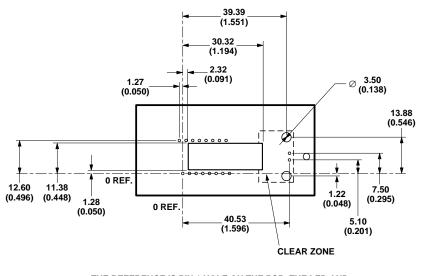
THE REFERENCE IS PIN 1 HOLE ON THE PCB. THE LED AND CLIP HOLES ARE HELD TO THIS DIMENSION TO  $\pm$  0.1 mm.
