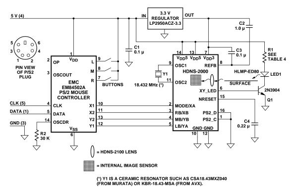
Figure 8. Typical Application using Quadrature Output Interfacing to PS/2 Mouse Controller.
