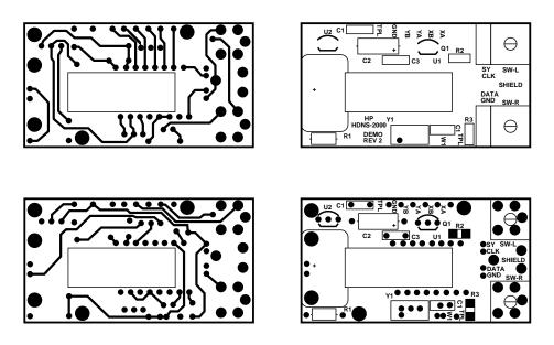
NOTE: AGILENT RECOMMENDS THAT THE COMPONENTS BE PLACED SO THEY ARE NOT IN THE AREA OF THE LENS RIDGE.
