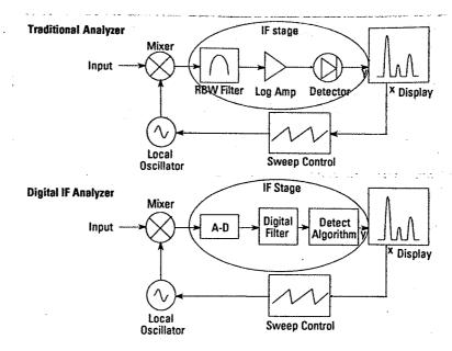
Figure 1: The digital IF analyzer replaces the analog RBW filter with a digital filter that offers more predictable noise bandwidth. The log amplifier and envelope detector are replaced by a digital algorythm that computes average power that provides accurate detection for both CW signals and noise.
