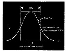
Figure 4: Noise power bandwidth is defined by an ideal filter that has the same area as the actual filter in the analyzer.
