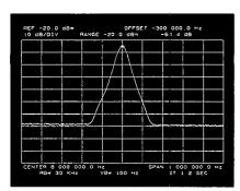
Figures 10A and 10B:The 17 kHz bandwidth on the HP 3588A (10A) produces the same result as an uncorrected measurement made in a 30 kHz bandwidth on a traditional analyzer like the HP 3585A (10B).
