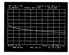
Figures 6A and 6B: The 17 kHz filter in the HP 3588A (6A) produces the same result as the 30 kHz filter in traditional analyzers like the HP 3585A (6B).
