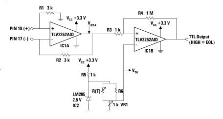
Figure 3. Laser bias indicator interface circuit
