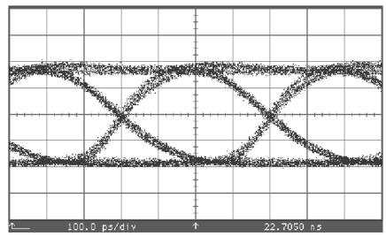
Figure 1(a). Typical HFCT-5942L transmitter output
