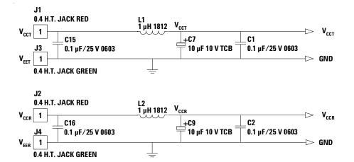
Figure 17. Filter Network for Power Supply Noise Reduction
