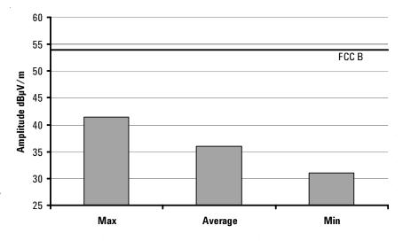
Figure 18. Radiated emissions for HFCT-5942L/AL
