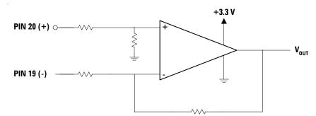
Figure 6. Rear facet monitor interface circuit. Resistor network should be used to reflect the gain required by the interconnecting IC and the output range of the product being used.
