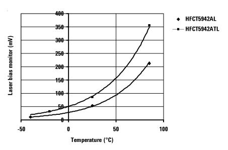
Figure 4. Typical variations of laser bias monitor voltage over temperature
