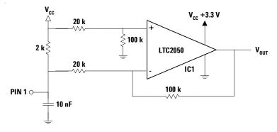
Figure 10. Photo detector bias current interface circuit
