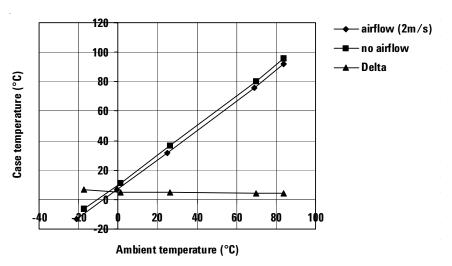
Figure 14(b). Case temperature variations as a function of ambient temperature under airflow (2 m/s)/and no airflow conditions
