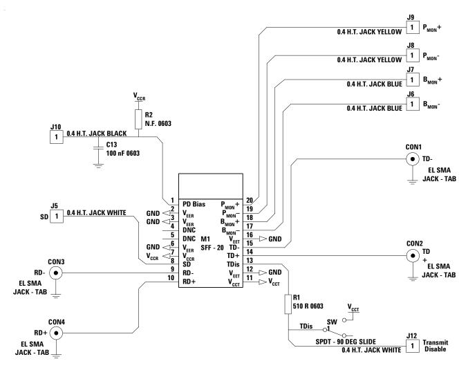
Figure 16. SFF Test Fixture Circuit Diagram for 2.5 Gb/s Transceivers
