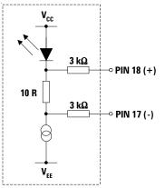
Figure 2. Bias monitor circuit (internal)
