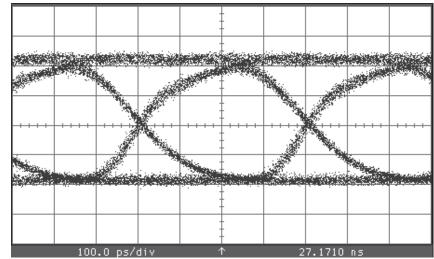
Figure 1(b). Typical HFCT-5942TL transmitter output
