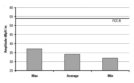
Figure 19. Radiated emissions for HFCT-5942TL/ATL
