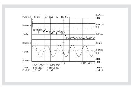
Figure 24. Display of the demodulated jitter spectrum and waveform
