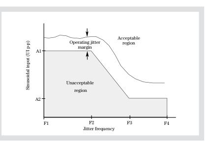
Figure 3. Jitter tolerance template
