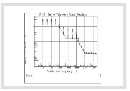
Figure 15. Results of jitter tolerance test
