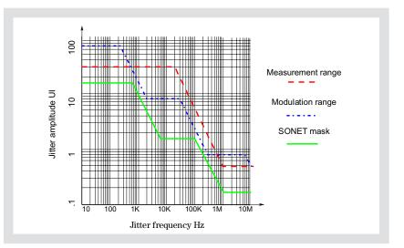
Figure 11. Jitter measurement characteristics (rate: 2.48832 Gb/s)
