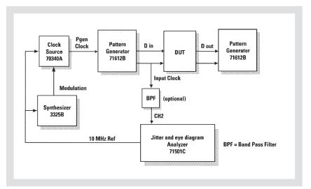
Figure 13. Setup for jitter tolerance measurement
