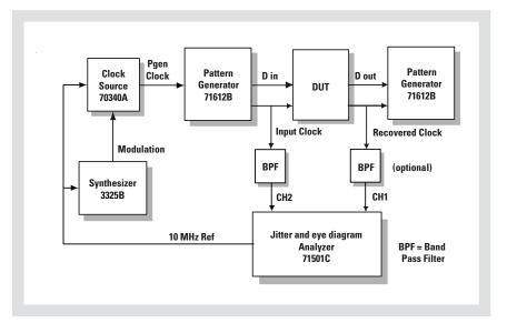
Figure 28. System configuration for 100 Mb/s to 12 Gb/s
