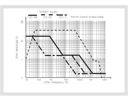
Figure 30. 70340A clock source modulation capability
