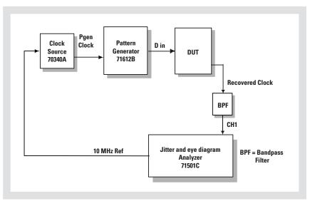
Figure 20. Setup for intrinsic jitter measurement
