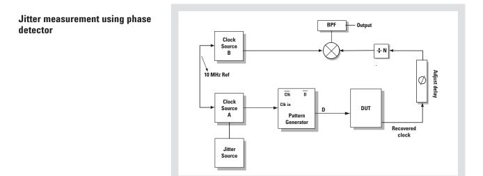
Figure 8. Configuration when using a phase detector
