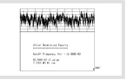
Figure 21. Example results for jitter generation measurement
