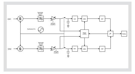
Figure 23. Block diagram of 71501C analyzer
