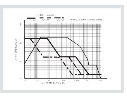
Figure 31. 83752A clock source modulation capability
