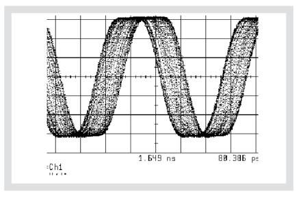
Figure 26. Display of clock waveforms with jitter
