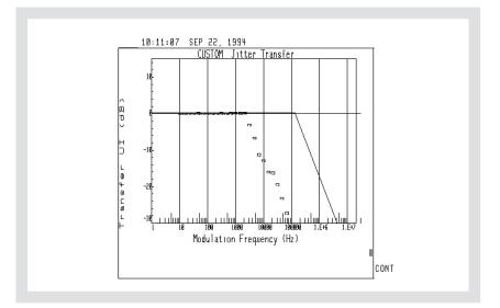
Fig 19. Results for custom jitter transfer measurement
