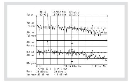
17. Example jitter transfer measurement
