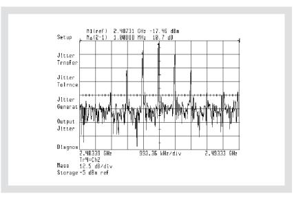
Figure 25. Display of sinusoidal jitter modulation present on the clock
