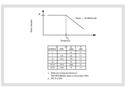
Figure 5. Jitter transfer specification
