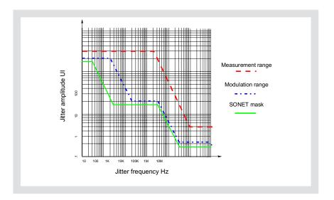
Figure 12. Jitter measurement characteristics (rate: 622.08 Mb/s)
