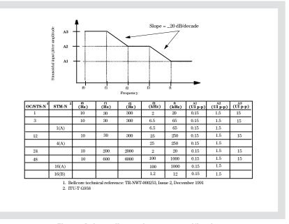
Figure 4. Input jitter tolerance specification
