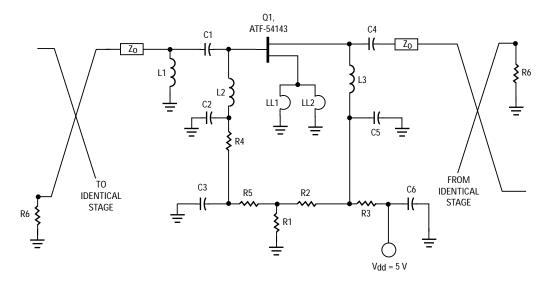
Figure 4. The Amplifier Schematic
