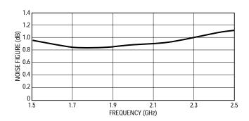
Figure 6. Linear Simulated Noise Figure vs. Frequency
