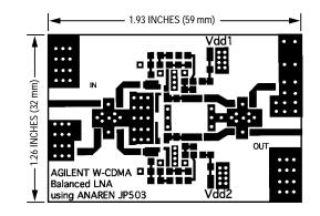
Figure 10. Artwork for the Balanced ATF-54143 Low Noise Amplifier
