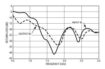
Figure 8. Linear Simulated Input and Output Return Loss vs. Frequency
