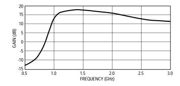
Figure 7. Linear Simulated Gain vs. Frequency
