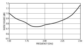
Figure 14. Noise Figure vs. Frequency
