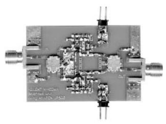
Figure 12. Photograph of Balanced Amplifier Board
