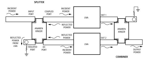
Figure 3. A Balanced Low Noise Amplifier
