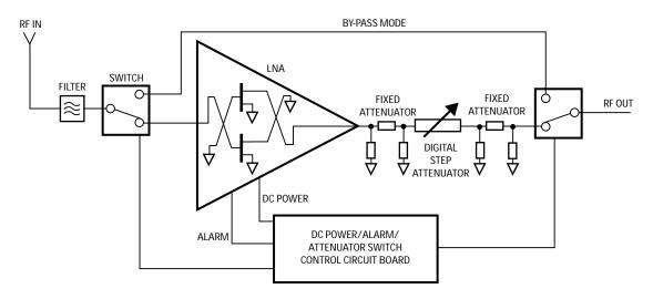
Figure 1. Tower Mounted Amplifier Functional Block Diagram
