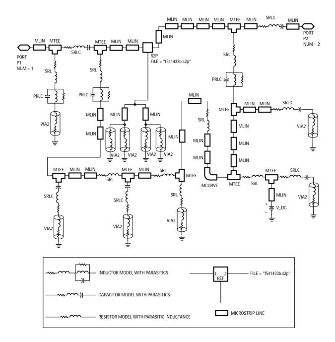
Figure 5. ADS Schematic
