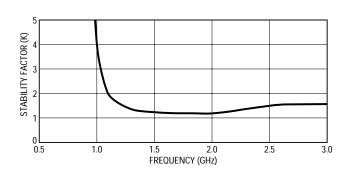
Figure 9. Simulated Rollett stability factor K
