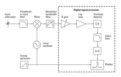
Figure 2. Block diagram of a superheterodyne spectrum analyzer
