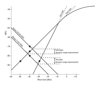
Figure 13. Reducing resolution bandwidth improves dynamic range
