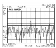
Figure 11. Using limit lines to detect spurious signals
