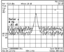
Figure 16. Externally generated distortion products
