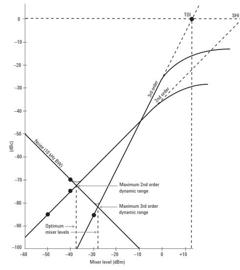
Figure 12. Dynamic range versus distortion and noise
