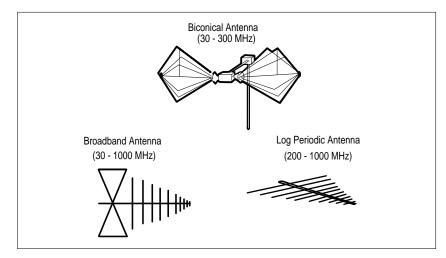
Figure B-2. Antennas used in EMI emissions measurements.
