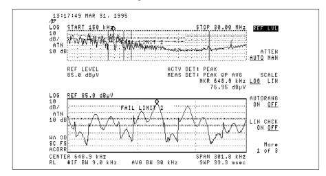
Figure 9. Conducted emissions from EUT in log format.
