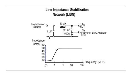
Figure A-1. Typical LISN circuit diagram.
