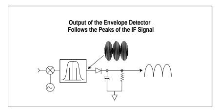
Figure D-1. Peak detector diagram.
