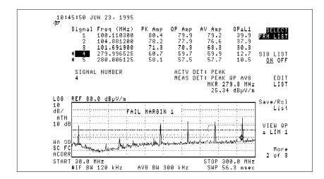
Figure 15. Measurements list compared to limit.
