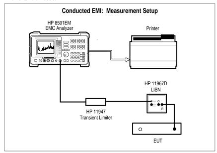
Figure 4. Conducted measurements interconnection.
