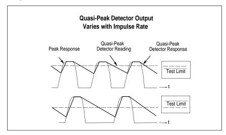
Figure D-2. Quasi-peak detector response diagram.
