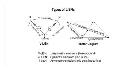
Figure A-2. Three different types of LISNs.
