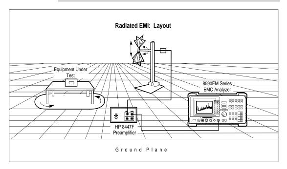
Figure 11. Radiated emissions test setup.
