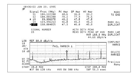
Figure 14. Radiated emissions measurement list.
