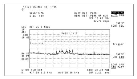
Figure 8. Noise picked up by power cord with EUT off.
