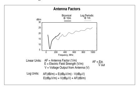
Figure B-1. Typical antenna factor shapes.
