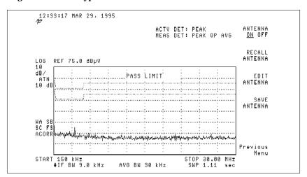
Figure 6b. Display corrected for LISN factors.
