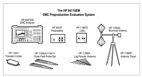
Figure 3. Components of a preproduction evaluation system.
