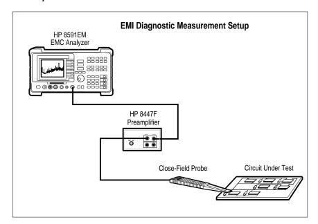
Figure 17. Diagnostics setup interconnection.
