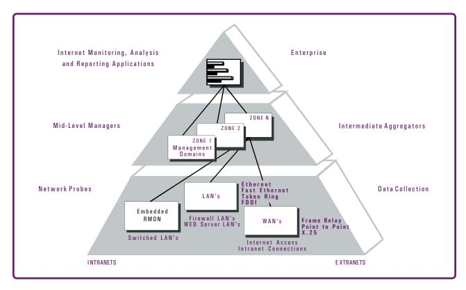
Figure 6: NetMetrix Distributed Architecture
