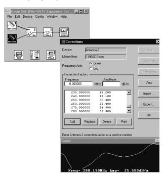
Figure 24: The 85876B can set up your equipment and import correction factors to correct for your measurement path.
