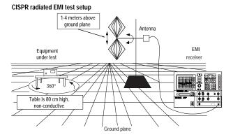
Figure 14: Radiated test setup
