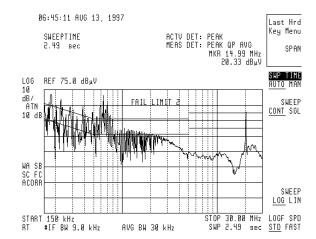
Figure 9: Log sweep for conducted test
