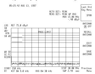
Figure 6: Display corrected for a LISN and limit lines on (no input connected to the receiver). The top limit is the quasi-peak limit and the bottom limit is the average limit.
