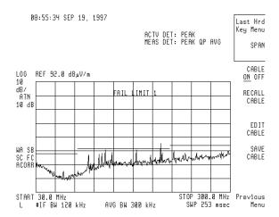
Figure 17: An ambient environment for radiated emissions. Ambients can often be above your limit line.
