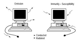
Figure 1. Two types of EMC measurements
