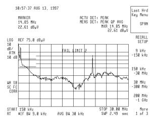
Figure 8: Conducted failure
