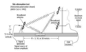
Figure 13: NSA procedure schematic, horizontal polarization
