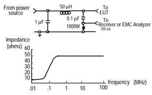
Figure A-1. Typical LISN circuit diagram
