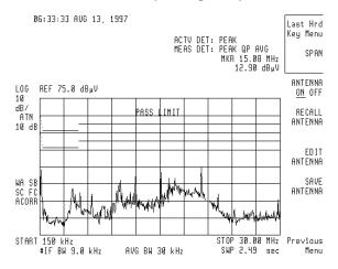
Figure 7: A conducted test in an ambient environment
