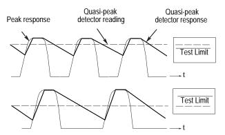
Figure D-2. Quasi-peak detector response diagram
