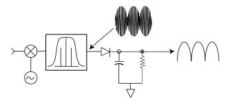
Figure D-1. Peak detector diagram
