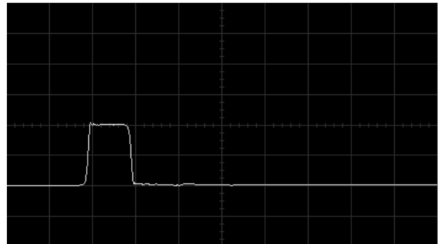
Figure 7b. Screen capture of short circuit termination from HP 54750A
