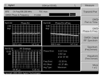
Figure 7. Quad display of the Agilent E4440A PSA series spectrum analyzer showing GMSK modulation metrics graphics of phase error with and without frequency error
