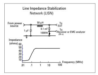
Figure A-1. Typical LISN circuit diagram
