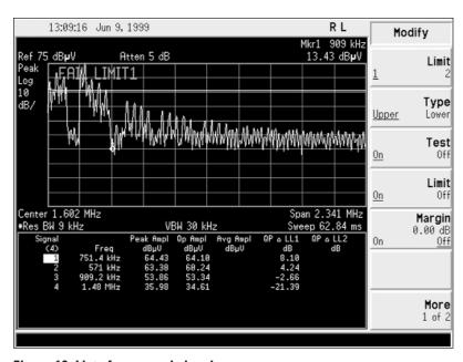
Figure 10. List of measured signals
