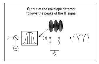
Figure D-1. Peak detector diagram
