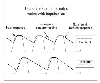
Figure D-2. Quasi-peak detector response diagram
