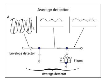
Figure D-3. Average detection response diagram
