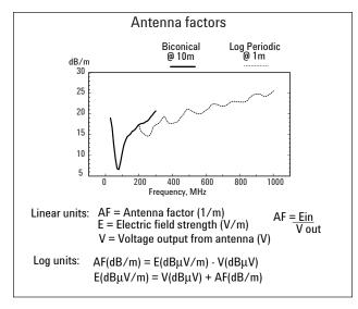
Figure B-1. Typical antenna factor shapes
