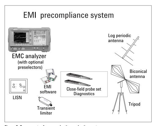
Figure 3. Components of a preproduction evaluation system
