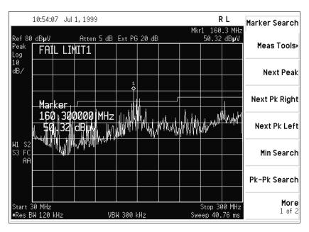
Figure 13. Radiated emissions display
