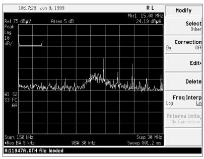
Figure 7b. Display corrected for limiter losses
