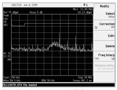
Figure 8. Noise picked up by power cord with EUT off
