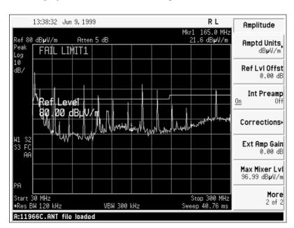
Figure 12. Display with limit line and correction factors
