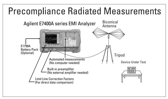
Figure 11. Radiated emissions test setup
