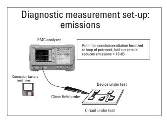
Figure 16. Diagnostics setup interconnection
