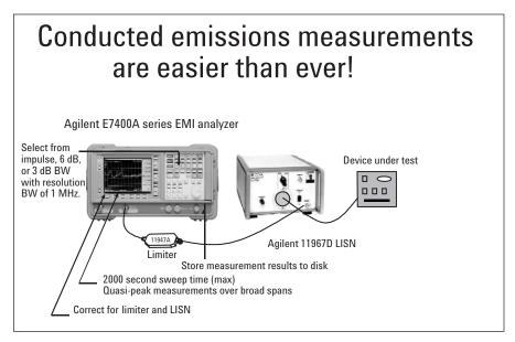
Figure 4. Conducted measurements interconnection
