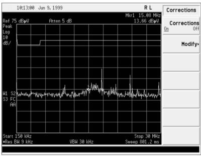
Figure 6b. Display corrected for LISN factors
