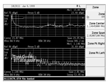
Figure 9. Conducted emissions from EUT
