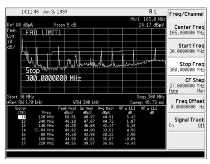
Figure 14. Measurements list compared to limit
