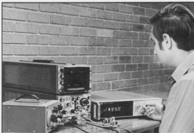
Low frequency square wave amplitude measurements being made using the 3480A Multifunction Digital Voltmeter and the 180A Oscilloscope.
