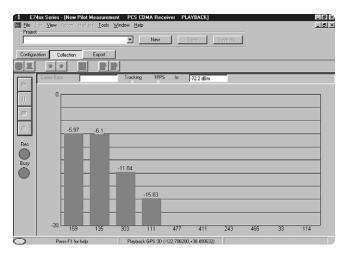
Figure 7. Receiver-based drive test measurement display of the four highest-level pilots.
