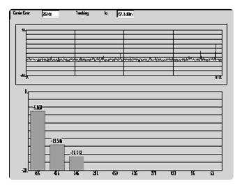
Figure 16. Properly optimized network. Receiver display indicates that pilot pollution is not present. Both the All Pilots and Top N displays are shown.
