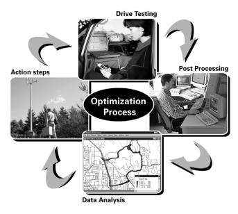
Figure 2. Optimization process begins with drive testing, moves to post-processing, then requires data analysis, and finally action needs to be taken to correct the problems. Drive-testing is performed again to verify that the actions were effective.
