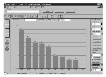
Figure 18. Absolute timing delay measurement using receiver-based system.
