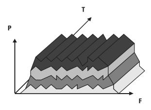
Figure 5. CDMA spectrum occupies 1.25-MHz bandwidth and consists of multiple code-domain channels, rather than individual narrowband frequency channels that were used in analog FM systems.
