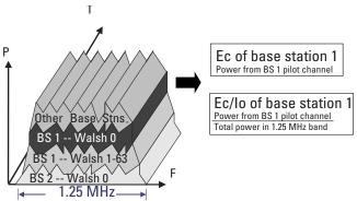
Figure 9. CDMA composite signal consisting of all the Walsh codes of each base station.
