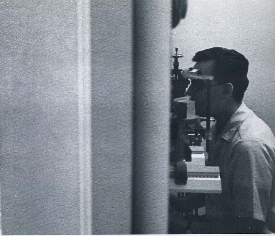
The department's computer controls apparatus in a visual perception lab and measures and records a subject's responses.
