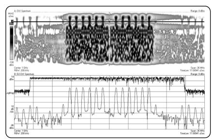
Figure 3.3.6: Spectrogram analysis of an OFDM burst
