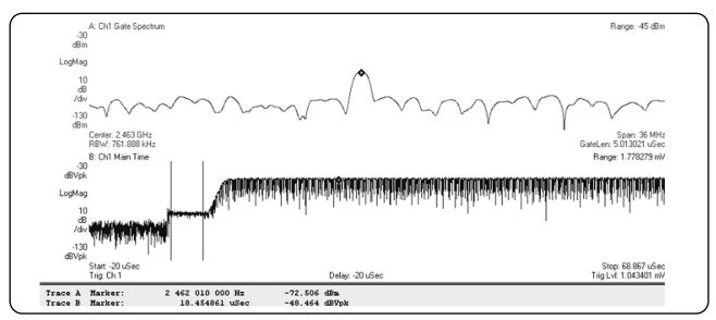
Figure 2.3.4: Investigating anomalies in a power burst through gated spectrum analysis
