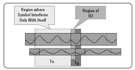
Figure 3.2.4: Guard interval and signal interactions
