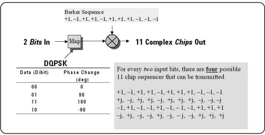
Figure 2.1.2: DSSS signal spreading for 2 Mbit/sec data rate
