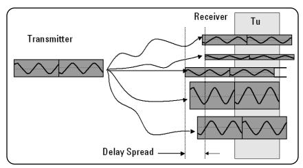
Figure 3.2.2: Effects of multipath delay
