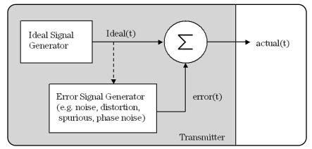
Figure 2.3.12: Signal error model
