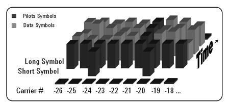
Figure 3.3.5: 802.11a carrier assignments.
