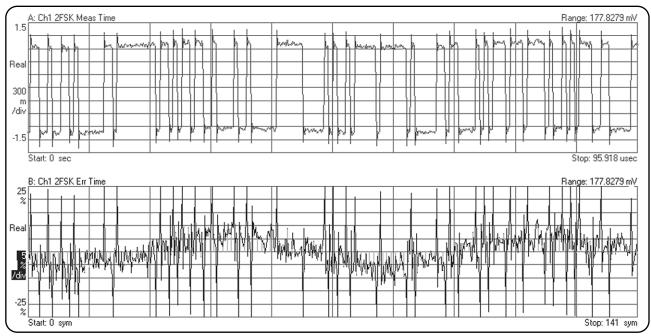
Figure 1.1.3: Residual FM on a FSK waveform
