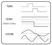
Figure 3.1.1: Orthogonal signals
