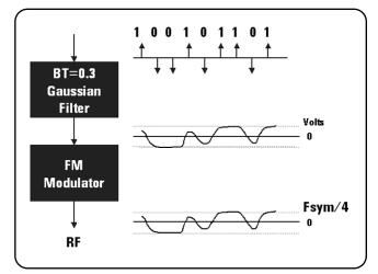
Figure 1.2.1: GMSK modulation method 1
