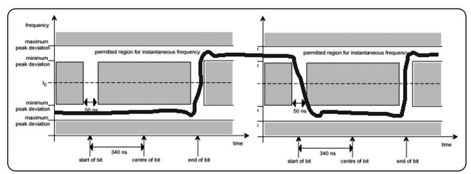
Figure 1.1.2: Eye-diagram mask for low-rate FSK modulation
