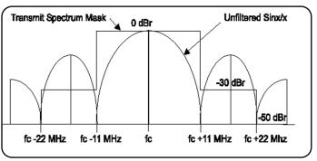
Figure 2.3.7: 802.11b transmit spectral mask
