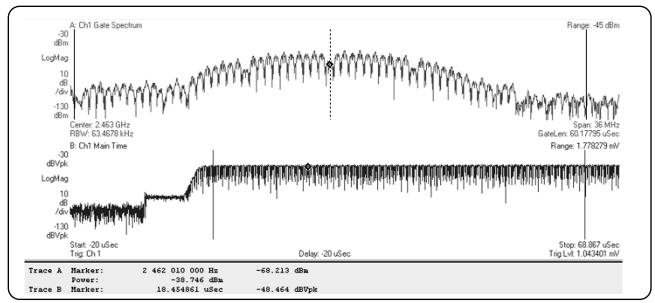
Figure 2.3.3: Gated spectrum analysis of power-up of an 802.11b signal
