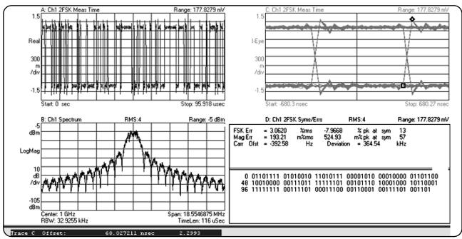
Figure 1.1.1: 2-FSK signal characteristics
