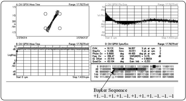
Figure 2.3.11: Demodulation of an 802.11b preamble
