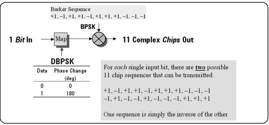
Figure 2.1.1: DSSS signal spreading for 1 Mbit/sec data rate
