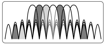
Figure 3.1.2: OFDM carrier separation
