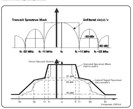
Figure 3.1.3: Transmit spectrum mask for 802.11a
