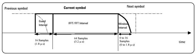
Figure 3.2.5: Windowing of OFDM symbols to reduce out-of-band power
