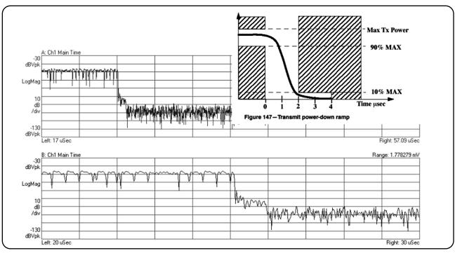
Figure 2.3.6: 802.11b power-down-envelope mask
