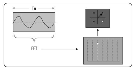
Figure 3.2.1: Receiving an OFDM signal
