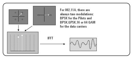
Figure 3.1.7: IFFT used to create multiple carriers
