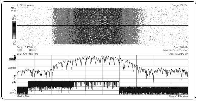
Figure 2.3.9: Spectrogram analysis of a single 802.11b burst
