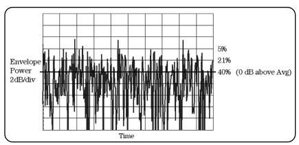
Figure 3.3.8: Power versus time for an OFDM burst
