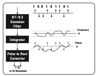
Figure 1.2.2: GMSK modulation method 2
