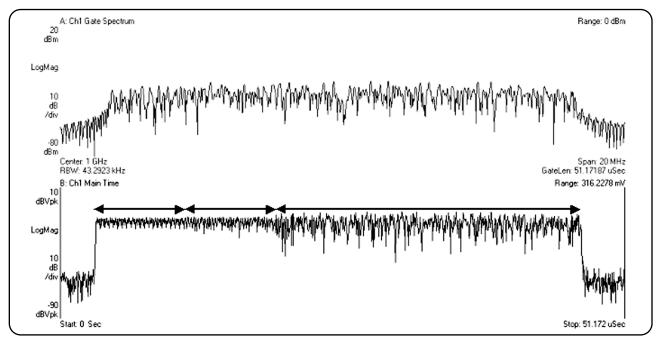
Figure 3.3.1: OFDM power burst and spectrum
