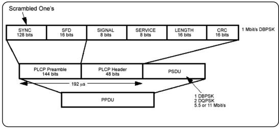
Figure 2.2.2: 802.11b PPDU components
