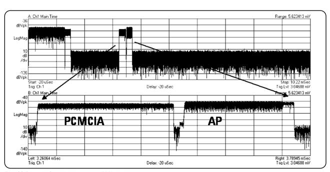
Figure 2.3.10: Analysis of an exchange between two WLAN modems  $\,$
