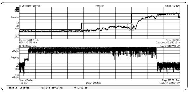
Figure 2.3.8: Signal analysis through gated sweep measurements
