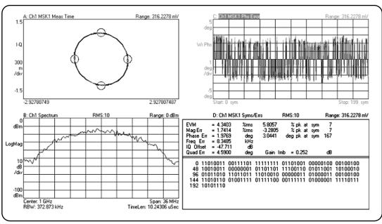
Figure 1.3.1: GMSK signal demodulation
