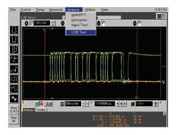
Figure 2. D+ and D- data signals are automatically bracketed by the Agilent Infiniium 54800 Series USB Test Option.
