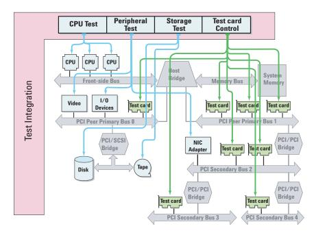
Figure 3. By using appropriate test cards, a single piece of software allows you to easily test very complex systems.
