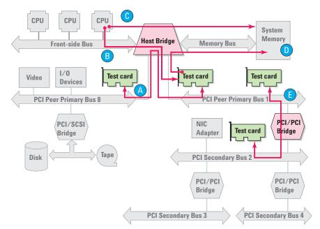
Figure 2. Using test cards, you can generate data traffic along any data path that is accessible by a connector. A bridge can be tested and stressed by placing two cards on either side of the bridge.
