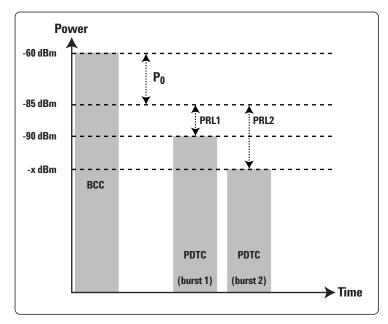
Figure 5. Setting up power offsets and reduction levels
