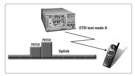
Figure 6. Diagram of ETSI test mode A connection
