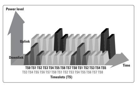
Figure 1b: Burst offset arrangement in GPRS
