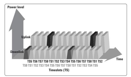
Figure 1a. Burst offset arrangement in GSM
