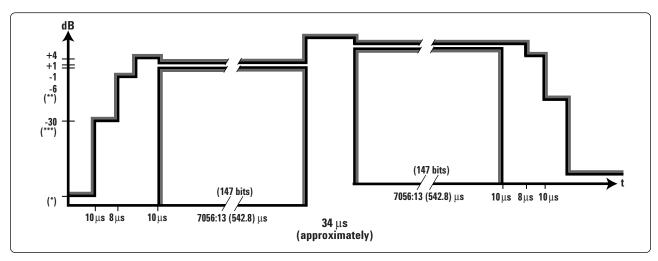
Figure 3. Specification for uplink power vesus time mask
