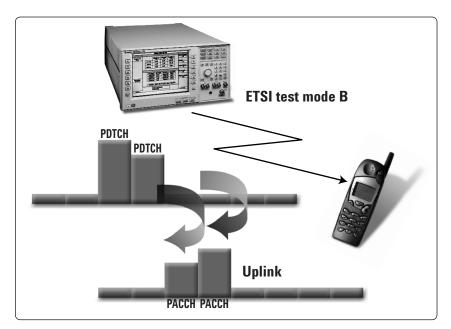
Figure 7 Diagram of ETSI test mode B connection
