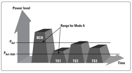
Figure 2. Period between bursts is only 34 µs
