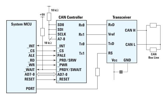
Figure 9. Example CAN node.
