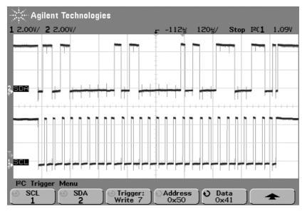
Figure 4. I<sup>2</sup>C trigger on a Write Frame with Address and Data. This powerful triggering feature allows the user to look within the I<sup>2</sup>C frame to trigger when a device at a particular address is written to or read from with a data value.
