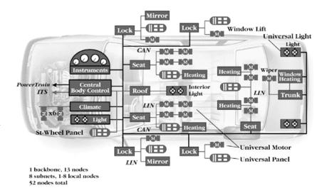
Figure 8. Example CAN automobile system. (Diagram courtesy of Motorola Inc.)
