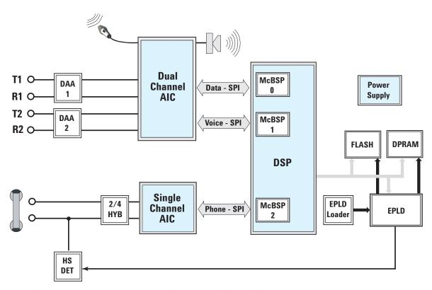
Figure 6. Web Phone Block Diagram; example of a multi-slave SPI bus, DSP-based system.
