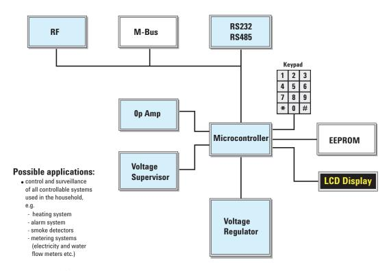
Figure 1. Example of a microcontroller-based design used to monitor and control devices in the home. The microcontroller uses the SPI bus to communicate with an RF tranceiver, an RS232 bridge, an EEPRPOM, a keypad, and display
