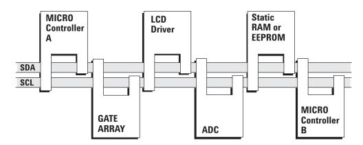
Figure 2. Example of an I<sup>2</sup>C bus system. The I<sup>2</sup>C bus consists of two active signals, SDA and SCL. Every component on the bus has its own unique address.
