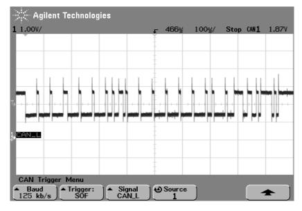
Figure 11. The user can specify the CAB-based signal to monitor. Shown here is a CAN-L signal.
