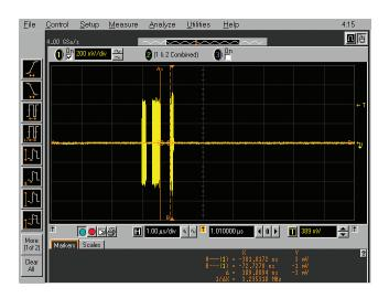
Figure 13. Device inter-packet gap.
