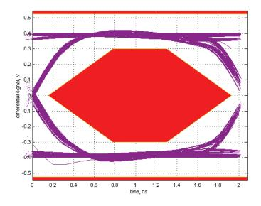
Figure 12. Hi-speed signal quality eye diagram.
