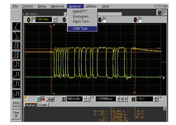
Figure 3. Captured downstream packet.
