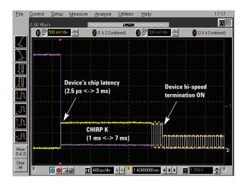
Figure 15. CHIRP test.
