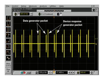
Figure 14. Receiver sensitivity test.
