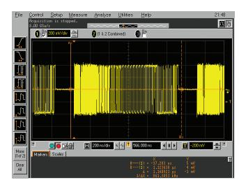
Figure 11. Hi-speed test packet.
