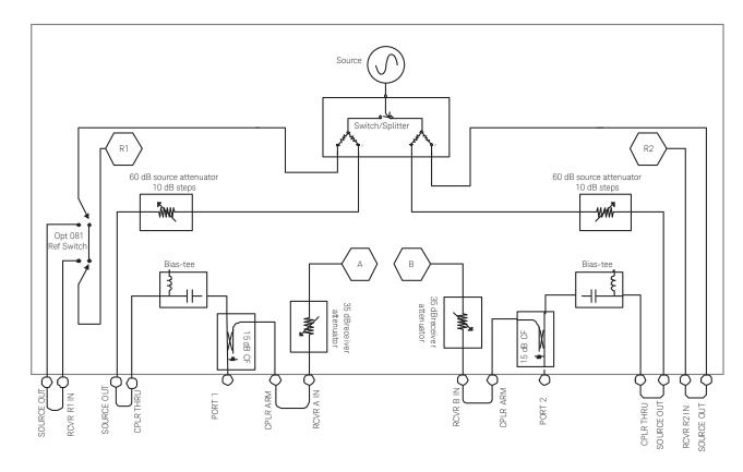
Figure 1. PNA (E8362/3/4B) block diagram for basic measurements
