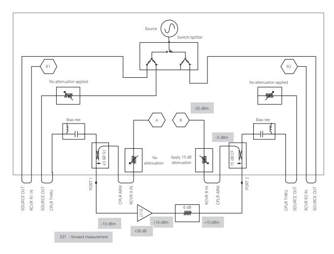
Figure 5. MW PNA E8364B for testing handset amplifier – low input power
