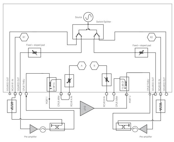
Figure 14. Two-way high-power measurements
