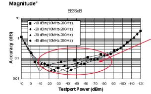
For best measurement accuracy, select the measurement and calibration power levels such that the test setup power levels remain in the relatively flat region.
