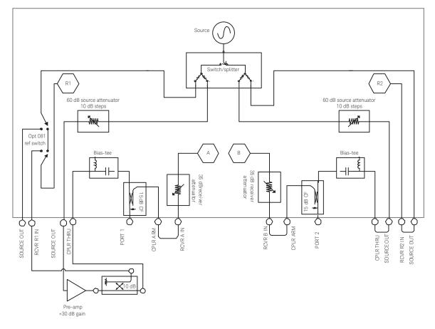
Figure 4. High-power setup connection diagram
