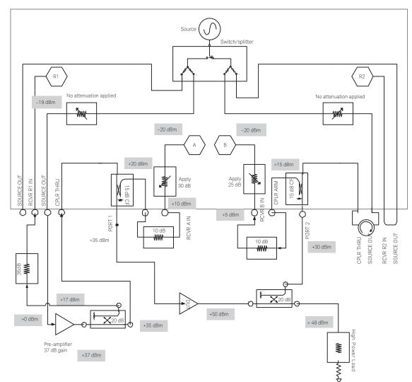
Figure 4. MW PNA E8362B-H85, configured to measure a solid state power amplifier
