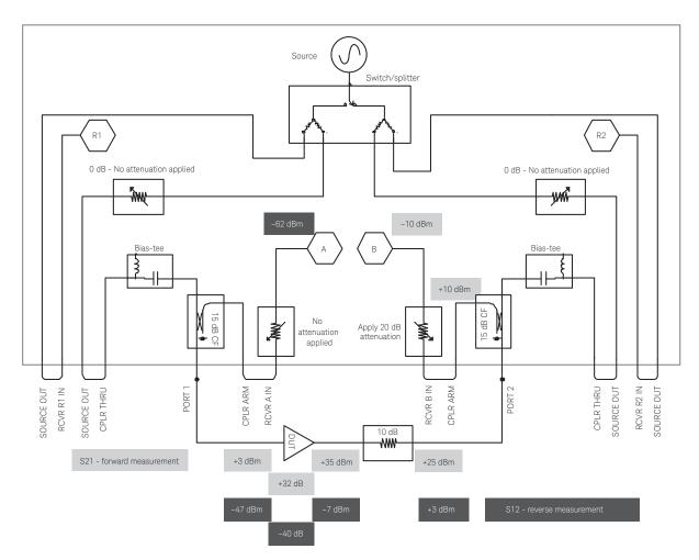
Figure 2. MW PNA E8362B, configured to measure a dual-band handset amplifier
