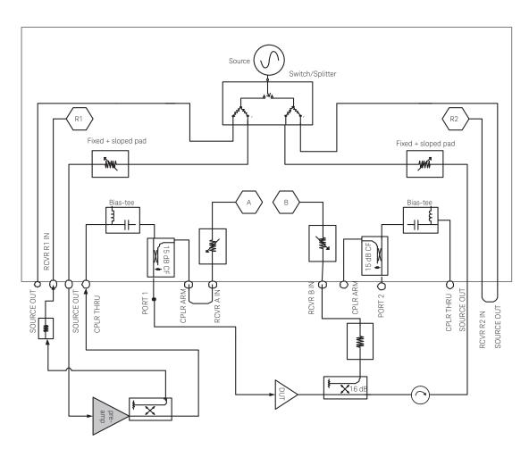
Figure 13. Use of external coupler in high-power measurements
