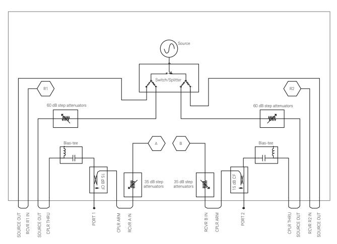
Figure 1. MW PNA E8362B block diagram, configured with source attenuators, receiver attenuators, bias-tees, and frequency-offset mode. (Options 016, UNL, 014, 080)
