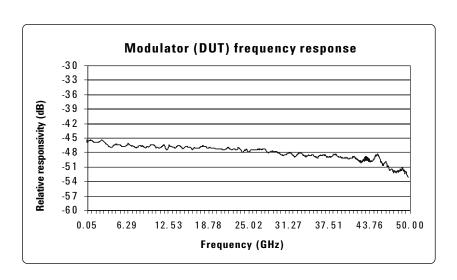
Figure 4. Measured optical modulator response using the PNA Series
