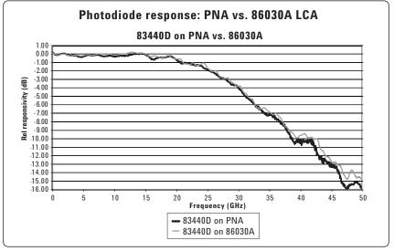
Figure 7. Measurement results as compared between the PNA Series and the 86030A LCA
