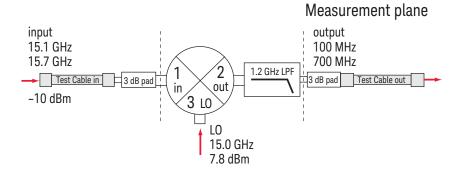
Figure 1. Example of a mixer-under-test configuration.
