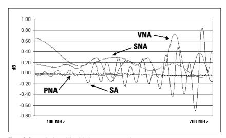
Figure 6. Conversion loss airline delta instrument comparison.
