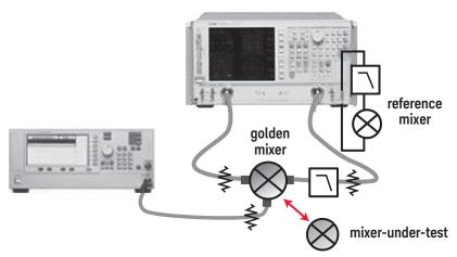
Figure 10. 8720ES group delay configuration using golden and reference mixers.
