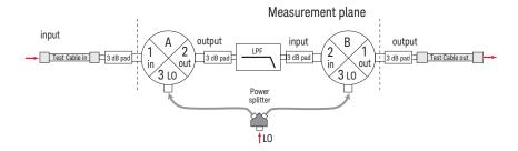
Figure 11. Up/down conversion method measures two mixers in series.
