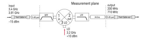
Figure 9. Converter configuration for airline delta comparison.
