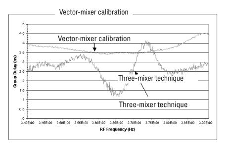
Figure 12. Measurement comparison of group delay techniques.
