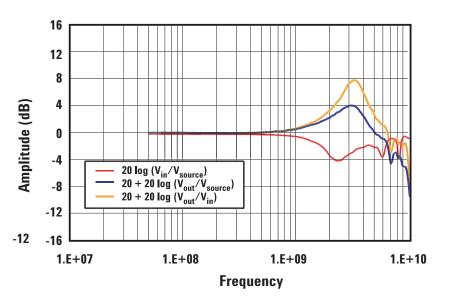
Figure 2. Six GHz "browser" probe equipped with socket accessory. Note +8 dB peaking at 3.3 GHz
