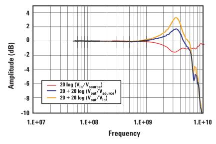
Figure 6a. Six GHz probe with fixed pin and pogo ground accessory. Even a stubby fixed pin causes +3 dB peaking at  $\sim$  3.5 GHz
