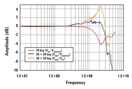
Figure 1. Traditional form factor 4 GHz probe with pin in signal socket and pogo pin in ground. Note >+4 dB peaking of V<sub>out</sub>/V<sub>in</sub> and 4 dB attenuation of V<sub>in</sub> at 2.25 GHz
