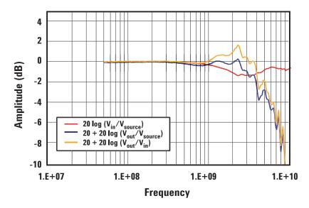
Figure 9. InfiniiMax single-ended solder-in probe head. Bandwidth is  $\sim$  5 GHz
