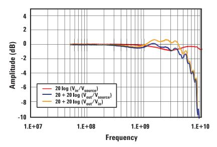
Figure 7b. InfiniiMax differential browser probe head with damped signal pins. Response is flat and V<sub>out</sub> tracks V<sub>in</sub>
