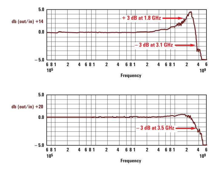
Figure 4a/b. Probe frequency response. Upper graph (4a) shows poor probe with peaking. Lower graph (4b) shows good probe with flat response.
