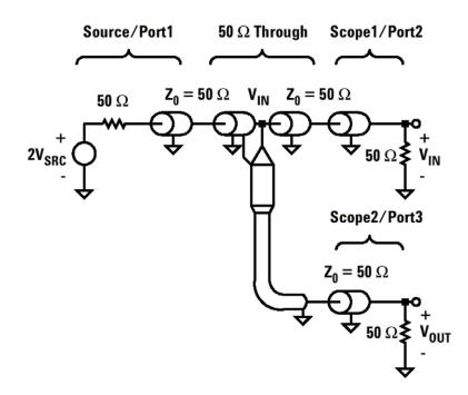
Figure 1. Setup to accurately measure a probe's input impedance and response.
