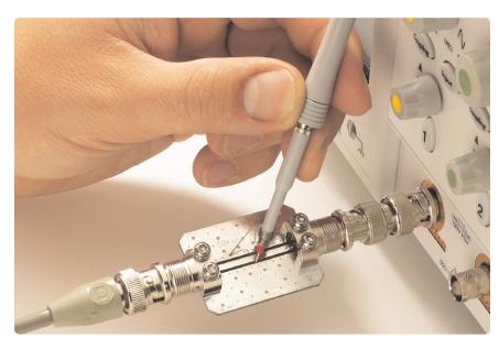
Figure 2. Fifty ohm through fixture, Agilent Technologies product number E2655-66501.
