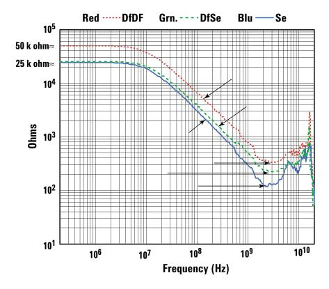
Figure 8. Input impedance of differential and single-ended probes
