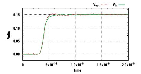
Figure 6. Time response of a single-ended probe to a 100 pS step
