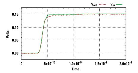
Figure 5. Time response of a differential probe to a 100 pS step
