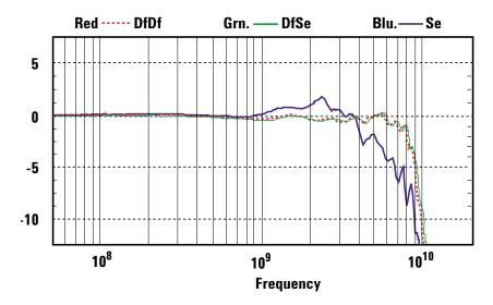
Figure 4. Frequency response of differential and single-ended probes
