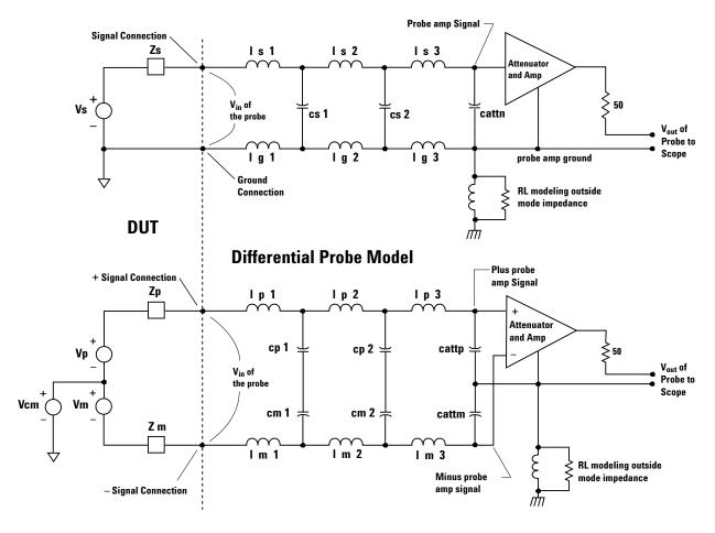
Figure 1. Simplified models of differential and single-ended probes
