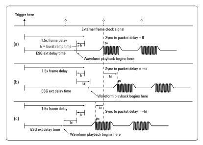
Figure 30: DH1 waveforms triggered from an external frame clock signal timing diagram. *NOTE:* The additional signals, illustrated with dotted arrows, the ESG receives during the playback of the dirty transmitter test sequence is ignored. When the playback of the sequence is completed, then the next trigger signal will start the playback of the next sequence.
