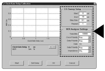
Figure 45. Clock/Gate Delay calibration utility setup.
