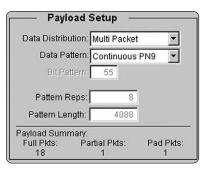
Figure 10. Payload Setup for a multi packet sequence with continuous PN9 user data.
