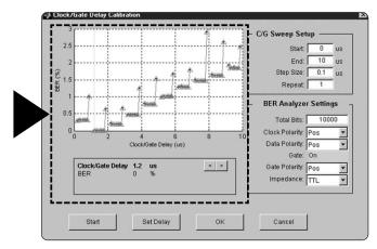
Figure 46. BER vs. Clock/Gate Delay calibration results.
