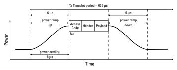
Figure 14. Burst profile of a single slot packet transmission with 6 µs power ramp and ramp settling.
