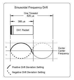
Figure 27. Sinusoidal carrier frequency drift impairment
