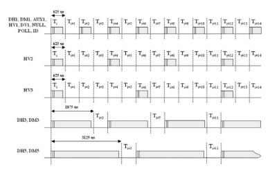
Figure 13. Bursted transmission timing relationships for different packet types.
