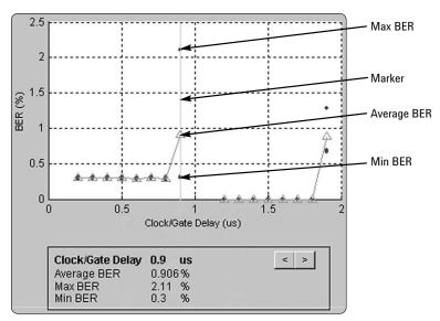
Figure 23. Plot of BER vs. Clock/Gate Delay with repetitions field set to three.
