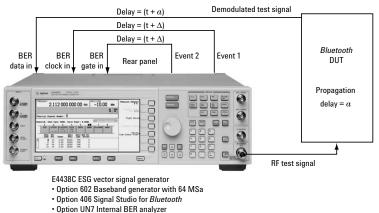
Figure 18. To perform BER analysis using this measurement setup, the clock/gate delay setting  $(\Delta)$  must be equal to the propagation delay the test signal experiences through the *Bluetooth* device (a).
