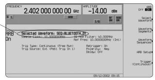
Figure 38. ESG dual arbitrary waveform generator user interface.
