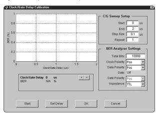
Figure 20. Clock/Gate Delay Calibration utility.
