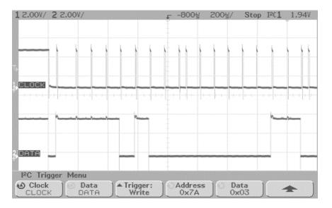
Figure 1. Setup for triggering an Agilent 54620 Series oscilloscope on the addressing of a 10-bit device with an address of 0x203 (1000000011<sub>2</sub>)
