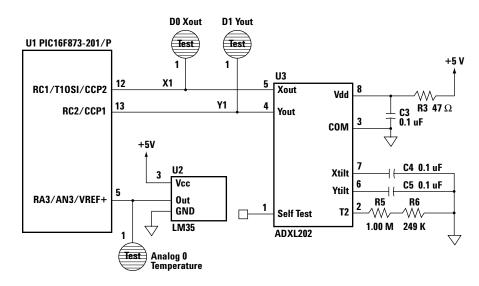
Figure 4. Basic diagram of the test setup.
