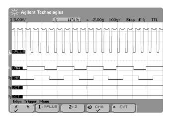
Figure 3. To verify that the encoder counts up when the motor is running forward, connect the 54642D MSO to the test points shown in Figure 2 and set the trigger for the rising edge of D2-CHA. You should see that D2-CHA leads the signal at D3-CHB, and that an up-count is present (a short logic 0) on D0-UCT.
