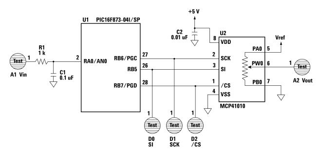
Figure 1. Simplified system diagram showing the filtered analog input to a PIC16F873, three digital lines connecting the PIC MCU to the MCP41010 digital pot, and the output of the pot. Two analog lines and three digital lines on the 54642D mixed signal oscilloscope monitor the system.
