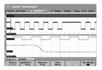
Figure 6. Verifying the clock frequency.
