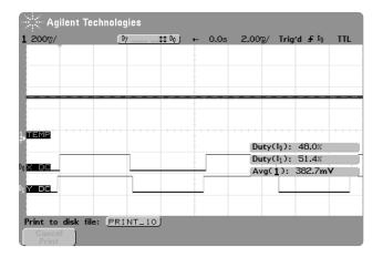
Figure 6. The 0 g bias when the room temperature is  $383 \text{ mv} / 10 \text{ mv}/\text{C} => 38\text{C}^{\circ}$
