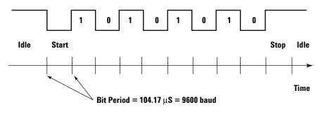
Figure 2. Representative serial byte.
