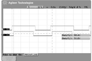
Figure 2a. X-axis sensitivity (Min and Max X duty cycles, Y at 0 g)
