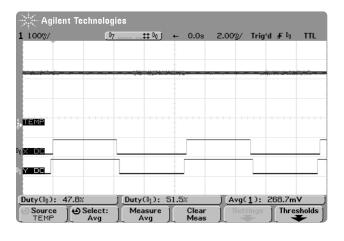
Figure 5. The 0 g bias when the room temperature is 269 mv / 10 mv/C => 27C°
