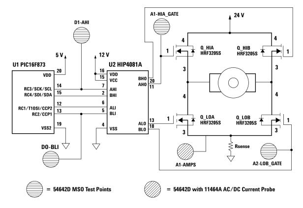
Figure 2. Basic diagram of the connections between the microcontroller, the level translation circuitry, and the four MOSFETS of the H-bridge.
