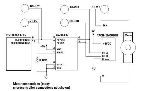
Figure 2. Schematic of a PIC18F252 microcontroller that converts up-counts and down-counts to position and velocity values.
