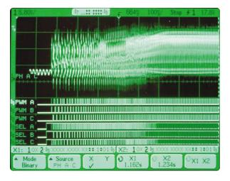
Figure 2. A high-resolution, analog-like display with 32-shades of gray helps you easily identify waveform irregularities (Agilent 54600 Series only).
