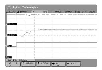
Figure 3. Using the "Quick Meas" menu in the 54642D MSO, the gate-drive voltage rise time can be quickly discerned.
