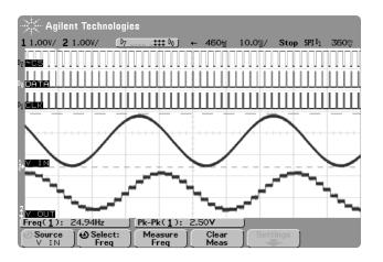
Figure 3. A sine wave screen showing the digital pot following an analog input.
