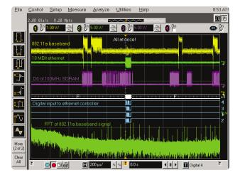
Figure 1. MegaZoom allows you to capture a full cycle of a device's operation while maintaining the ability to resolve fine details.
