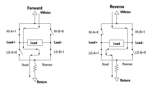
Figure 1. Logic state of the H-bridge transistors (1=on, 0=off) and the manner for turning them on and off to control motor direction.
