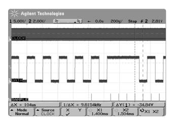
Figure 8. Showing the controller is measuring the bit period correctly.
