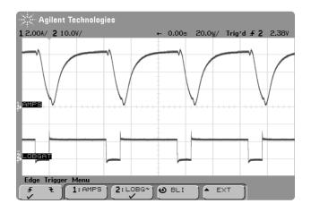
Figure 4. A measurement showing the motor current in relation to the low-side ( $Q_LOB$ ) MOSFET PWM control signal. With the 11464A AC/DC current probe set for 100 mV/Amp, the signals displayed show the expected current waveform. The 54642D MSO is set to trigger on the rising edge of the gate-drive signal of the MOSFETs.
