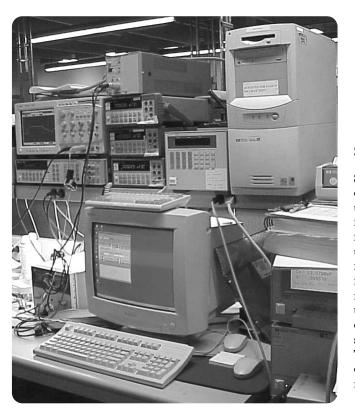
test and techniques such as using the same cables to increase repeatability, the manual approach can produce reasonably reliable results. Another advantage of manual control is the ease in which the test system can be reconfigured or the instruments used for other projects.
