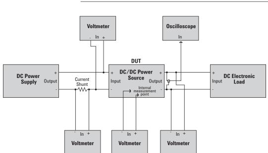
Figure 4 Block diagram of a manually controlled test system used for R&D
