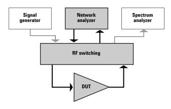
Figure 3. Network-analyzer paths to and from the DUT
