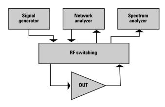
Figure 2. The essential elements of a simplified RF/microwave test system
