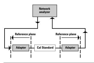
**Figure 4.** Adapter embedding moves the reference plane closer to the network analyzer, ensuring characterization of just the signal paths of interest
