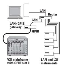
**Figure 2.** A router plus a LAN/GPIB gateway enables creation.
