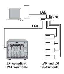
**Figure 5.** An LXI-compliant mainframe brings the benefits of PXI switching to a hybrid PXI/LXI system.
