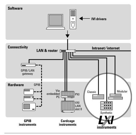
Figure 7. With Agilent Open and LXI, LAN becomes the backbone of test systems that easily incorporate present and future test assets.
