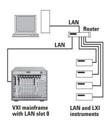
Figure 3. Add a LAN slot-0 card to a VXI mainframe to create a LAN-based hybrid VXI/LXI system.
