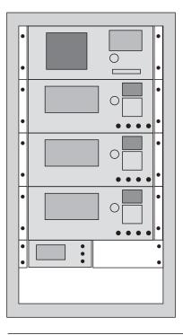
Figure 2. Redundant or unneeded hardware such as instrument displays, keypads and digitizers add extra space and weight to rack-and-stack systems.
