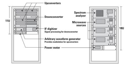
**System hardware:** As a comparison, a rack-and-stack system containing a spectrum analyzer, three microwave sources and a power meter might occupy 18U of rack space. Using a variety of half-rack SI modules that don't have displays or keypads, the same functionality occupies 11U of rack space, as shown in Figure 3. This type of system is smaller, lighter and easier to transport. It also simplifies support by making it easier to replace or upgrade individual instrument modules as needed.
