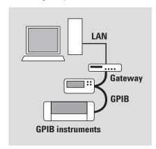
**Figure 2.** The test system configuration with the Gigabit Ethernet LAN switch
