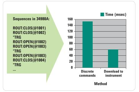
Figure 8. Internal management of switching and measurement within the 34980A switch/measure unit provides significant gains in speed.
