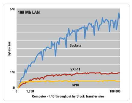
Figure 7. Sockets programming provides a significant speed advantage over GPIB and VXI-11.
