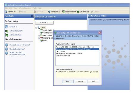
Figure 4. The Agilent Connection Expert utility can help you discover and connect GPIB instruments through the Agilent E5801A LAN/GPIB gateway.
