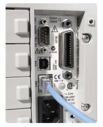
Figure 3. Many of today's instruments have multiple I/O ports: the Agilent 34980A switch/ measure unit shown here is equipped with GPIB, LAN and USB ports.
