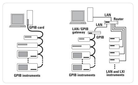
Figure 1. An all-GPIB system (left) can be easily converted to a hybrid structure (right).
