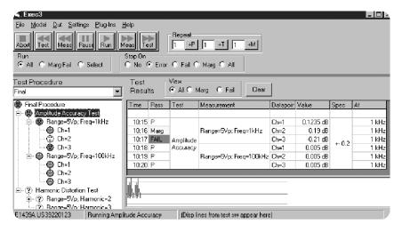
One of the most important features of a test executive is its test sequencer. As shown on the left side of Figure 11, the test sequencer is a sequence of tests that can be manipulated in design mode. Various test executives provide different levels of flexibility in this sequence, such as "test looping."
