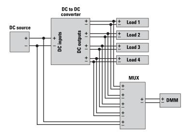
Figure 5. By using the built-in measurements in your DC power source and electronic loads, you can eliminate the DMM and MUX and significantly increase your test speed.
