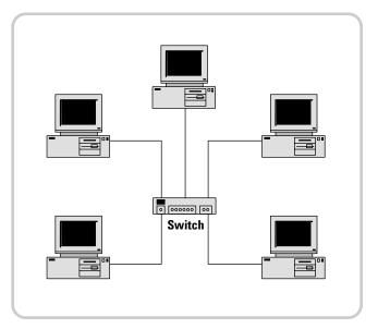
Figure 3. A simple network with one switch and multiple PCs in a star topology.
