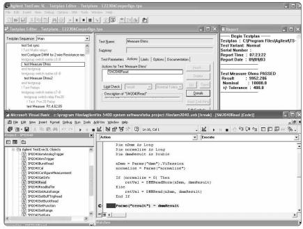
**Figure 2.** The main window of a typical test developer interface. The window frame on the left summarizes the hierarchical definition of the testplan. The middle frame displays details about the selected test. The right frame shows a summary of results from executing the testplan. Watch and Trace frames, used for debugging, are also displayed along the bottom. The entire screen presentation can be customized as desired.
