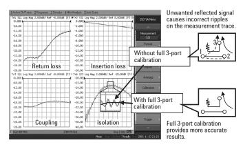
Figure 12. Full 3-port calibration in coupler measurement
