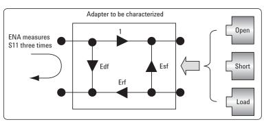
Figure 14. Adapter characterization (single directional method)
