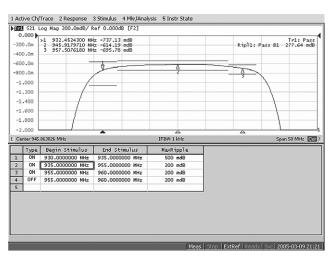
Figure 11. Ripple limit test
