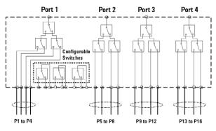
Figure 25-2. E5091A-016 16-port configuration block diagram
