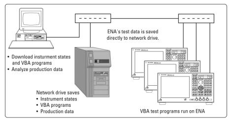
Figure 9. ENA factory automation example
