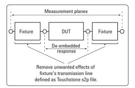
Figure 18. De-embedding for removing fixture effects
