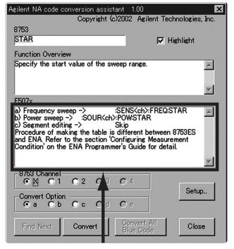
Figure 33. Quick Help shows equivalent GPIB commands and code conversion tips
