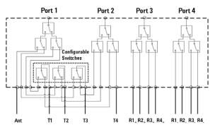
Figure 25-1. E5091A- 016 13-port configuration block diagram
