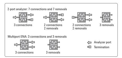
Figure 23. Number of connections/removals needed for duplexer test
