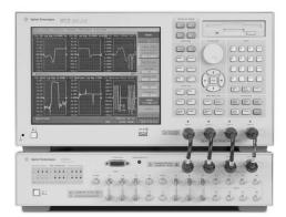
Figure 24. ENA and E5091A-016 test set
