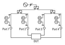
Figure 22. 4-port ENA hardware architecture
