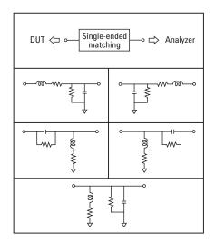
Figure 21. Pre-defined models of matching circuit embedding
