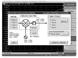
Figure 30. Vector-mixer calibration using VBA
