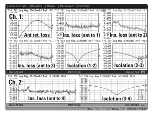
Figure 29. 4-way power divider measurement example using two full 4-port calibrations
