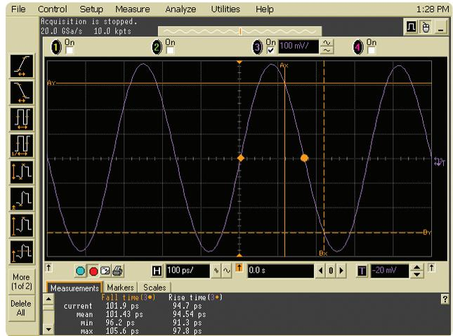
Figure 3. Rise/fall times on the Agilent scope
