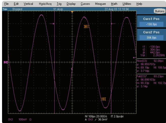
Figure 4. Rise/fall times on the Tektronix scope
