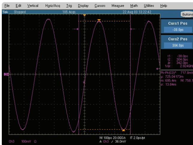
Figure 6.  $V_{\text{p-p}}$  measurement on Tektronix scope
