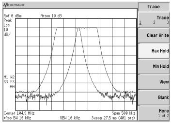
Figure 30. Peak-to-peak frequency deviation
