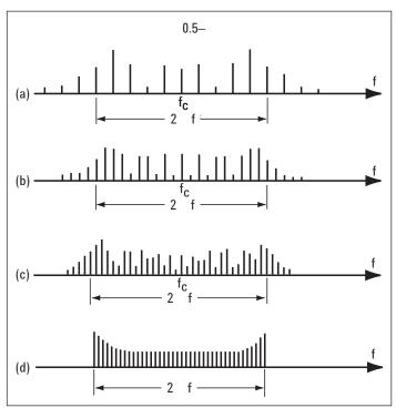
Figure 23. Amplitude-frequency spectrum of an FM signal (amplitude of delta f fixed; fm decreasing.) In (a),  $\beta$  = 5; in (b),  $\beta$  = 10; in (c),  $\beta$  = 15; in (d),  $\beta \rightarrow \infty$
