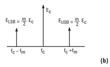
Figure 2(a)(b). Calculation of degree of amplitude modulation from time domain and frequency domain displays
