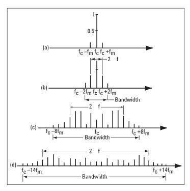
Figure 22. Amplitude-frequency spectrum of an FM signal (sinusoidal modulating signal; f fixed; amplitude varying). In (a),  $\beta$  = 0.2; in (b),  $\beta$  = 1; in (c),  $\beta$  = 5; in (d),  $\beta$ = 10
