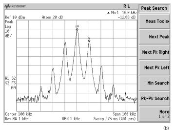
Figure 5. (a) An amplitude-modulated carrier in the time domain, (b) Shows the same waveform measured in the frequency domain
