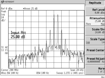
Figure 19. (a)A SSB generator, modulated with two sine-wave signals of 2000 and 3000 Hz. The 200 MHz carrier (display center) is suppressed 50 dB; lower sideband signals and intermodulation products are more than 50 dB down (b)The same signal after passing through an amplifier
