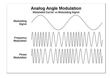
(2) Phase modulation can generally be converted into frequency modulation by choosing the frequency response of the modulator so that its output voltage will be proportional to 1/f<sub>m</sub> (integration of the modulating signal). The reverse is also true if the modulator output voltage is proportional to f<sub>m</sub> (differentiation of the modulating signal).
