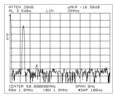
Figure 14. Using the FFT yields a frequency-domain display of just the modulation signal  $\,$
