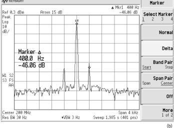
Figure 11. (a) Using markers to measure percent AM works well even at low modulation levels. Percent AM computed from ratio in A agrees with values determined from carrier/sideband ratio in (b)
