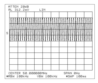
Figure 13. Sweep time adjusted to display many cycles
