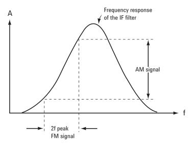
Figure 32. Slope detection of an FM signal
