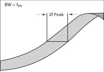
Figure 28. Measurement of fm and Δf<sub>neak</sub>
