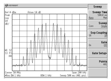
Figure 27. This is the spectrum of an FM signal at 50 MHz. The deviation has been adjusted for the first carrier null. The  $\rm f_m$  is 10 kHz; therefore,  $\Delta f_{\rm neak}$  = 2.4 x 10 kHz = 24 kHz
