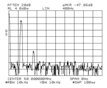
Figure 34. True distortion, using FFT to remove FM from the measurement
