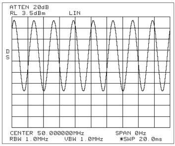
Figure 15. The modulation distortion of our signal cannot be read from this display
