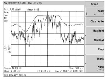
Figure 31. FM broadcast transmitter modulated with a stereo signal. 500 kHz span, 10 dB/div,  $\beta = 3$  kHz, sweeptime 50 ms/div, approx. 200 sweeps
