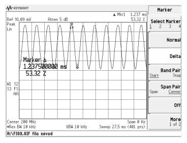
Figure 10. Delta markers can be used to find the ratio  $E_{min}/E_{max}$
