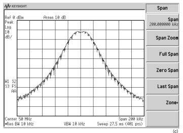
Figure 29. (a)A frequency-modulated carrier. Sideband spacing is measured to be 8 kHz (b)The peak-to-peak frequency deviation of the same signal is measured to be 20 kHz using max-hold and min-hold on different traces (c)Insufficient bandwidth: RBW = 10 kHz
