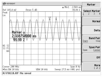
Figure 12. Time difference indicated by delta marker readout can be used to calculate frequency by taking the reciprocal
