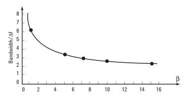
Figure 26. Bandwidth requirements vs. modulation index, ß
