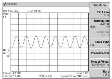
Figure 9 Placing the maxiima and minima on graticule lines makes the calculation easier
