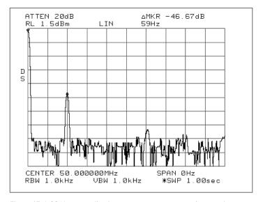
Figure 17. A 60 Hz power-line hum measurement uses a 1-second sweep time
