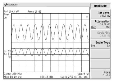
Figure 8. Moving the signal up and down on the screen does not change the absolute difference between Emax and Emin, only the number of display divisions between them due to the change of display scaling
