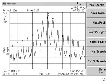
Figure 6. (a)An overmodulated 60 MHz signal in the time domain, (b) The frequency domain display of the signal
