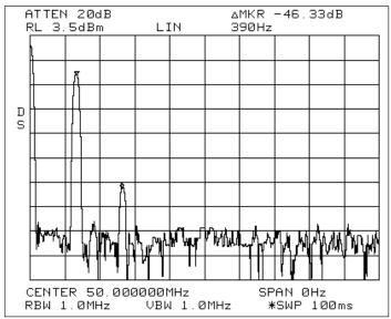
Figure 16. An FFT display indicates the modulation distortion; in this case, about 0.5% second-harmonic distortion
