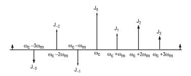
Figure A-5. Composition of an FM wave into sidebands
