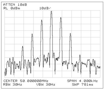
Figure 33. Pure AM or FM signals always have equal sidebands, but when the two are present together, the modulation vectors usually add in one sideband and subtract in the other. Thus, unequal sidebands indicate simultaneous AM and FM. This CW signal is amplitude modulated 80% at a 10 kHz rate. The harmonic distortion and incidental FM are clearly visible.
