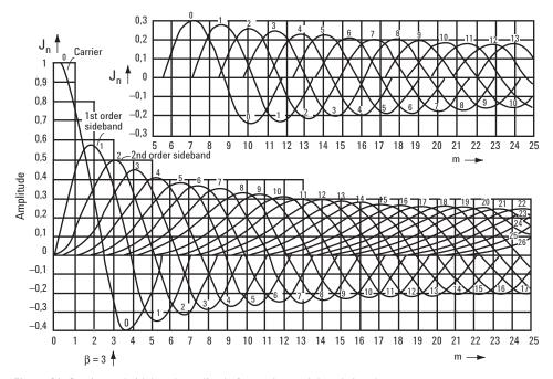
Figure 21. Carrier and sideband amplitude for angle-modulated signals
