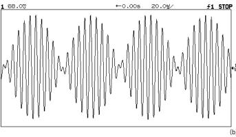
Figure 18. Frequency (a) and time (b) domain presentations of balanced modulator output
