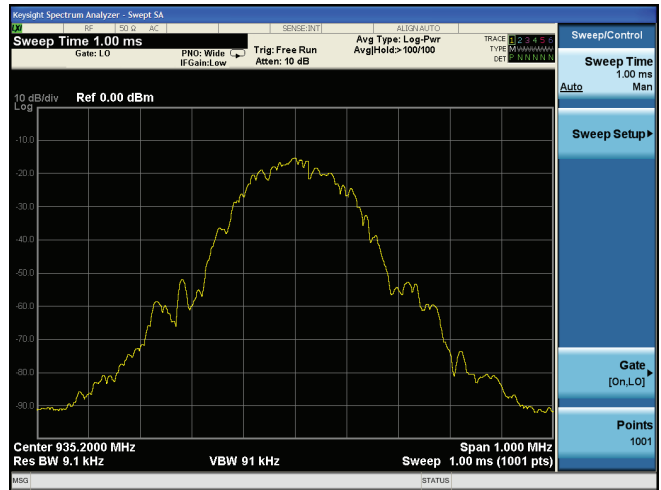
Figure 2-39. Spectrum of time slot 3 reveals that the spurious signal is not caused by this burst.
