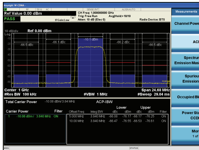
Figure 6-9. Adjacent channel power measurement using a PXA spectrum analyzer
