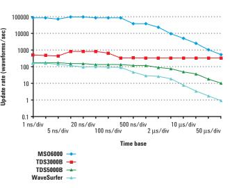
Figure 8. Waveform update rates using each scope's default real-time sampling mode.
