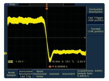
Figure 3. The Tektronix TDS3000B Series scope fails to capture the metastable state after 10 seconds of acquisition time.
