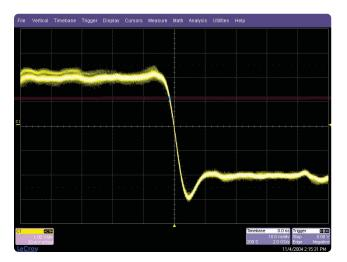
Figure 5. The LeCroy 400 Series scope fails to capture the metastable sate after 10 seconds using real-time sampling.
