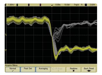
Figure 1. Infrequent metastable state captured on Agilent's MS06000 Series oscilloscope using real-time sampling.
