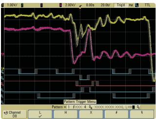
Figure 2. Pattern triggering reveals a setup-and-hold-time violation.
