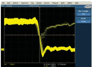
Figure 6. The Tektronix TDS5000B Series scope using FastAcq acquisition is able to capture the infrequent metastable using equivalent-time sampling.
