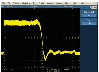
Figure 4. The Tektronix TDS5000B Series scope fails to capture the metastable state after 10 seconds using real-time sampling.
