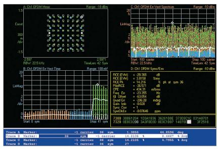
Figure 5. A basic digital demodulation result from the 89601A VSA measurement application including a constellation diagram and a composite table of error parameters and measured symbols, along with the two main error vector displays of error vs. time (lower left) and symbol and error vs. frequency (upper right). Marker coupling is used to correlate a peak in the error vector time trace across several displays and measurement domains.
