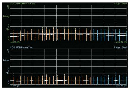
Figure 6. The magnitude portion of the error vector signal reveals the effect of pilot tracking. In the bottom trace amplitude tracking has been used, removing the amplitude drift which is evident in the top trace. Amplitude tracking improved the RCE (EVM) by about 5 dB.
