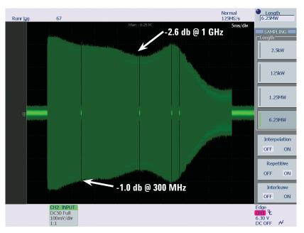
Figure 8: Swept frequency response test on a non-Agilent 1.5-GHz bandwidth scope
