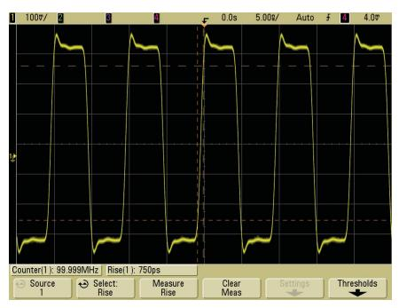
Figure 4: 100-MHz clock captured on the Agilent MS07054A 500-MHz bandwidth scope
