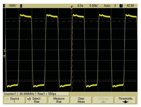
Figure 5: 100-MHz clock captured on the Agilent MS07104A 1-GHz bandwidth scope
