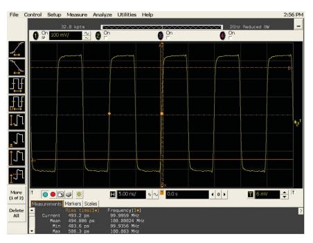
Figure 6: 100-MHz clock captured on the Agilent DS080204B 2-GHz bandwidth scope
