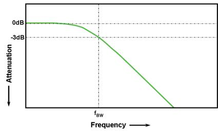
Figure 1: Oscilloscope Gaussian frequency response
