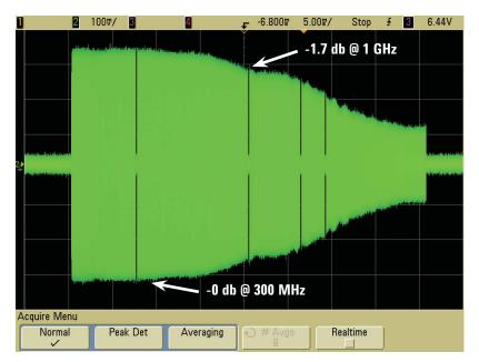
Figure 7: Swept frequency response test on Agilent's MS07104A 1-GHz bandwidth scope
