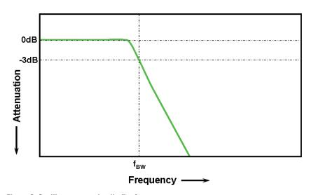
Figure 2: Oscilloscope maximally-flat frequency response
