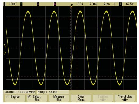
Figure 3: 100-MHz clock captured on the Agilent MSO6014A 100-MHz bandwidth scope
