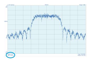
Figure 48. Spectrum of an IQ signal (QAM16)
