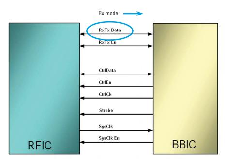
Figure 6. DigRF 1.12 interface between the RFIC and BBIC
