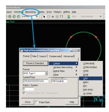
Figure 37. Selecting the modulation format
