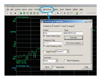
Figure 35. MeasSetup Properties dialog box
