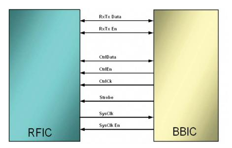
Figure 49. DigRF 1.12 ASIC interfaces
