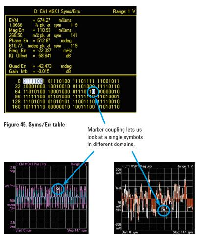
Figure 46. IQ phase error display
