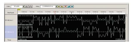
Figure 32. Waveform view in chart mode. In this mode, all the symbols are displayed as if they are in the time domain.
