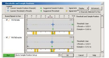
Eye finder shows the correct threshold, and the proper sample position.
