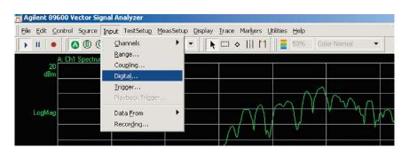
Figure 33. Drop-down menu for digital input properties
