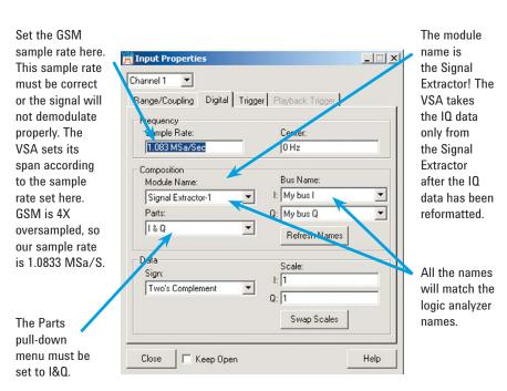
Figure 34. Digital Input Properties dialog box
