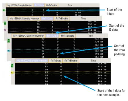
Figure 29. List view of pre-extracted data (serial). We can scroll down and count the bits using markers.
