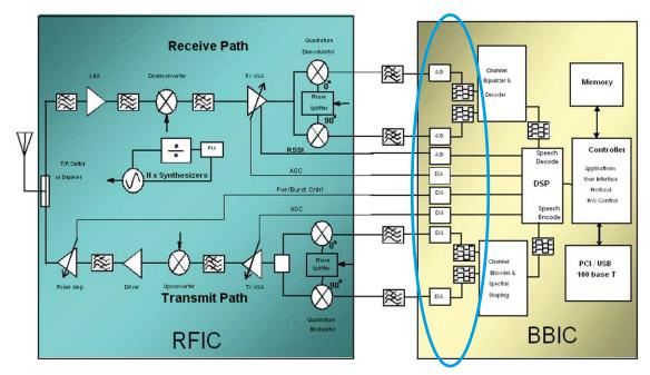
The ADCs used to be located in the BBIC and the chip interface was analog.
